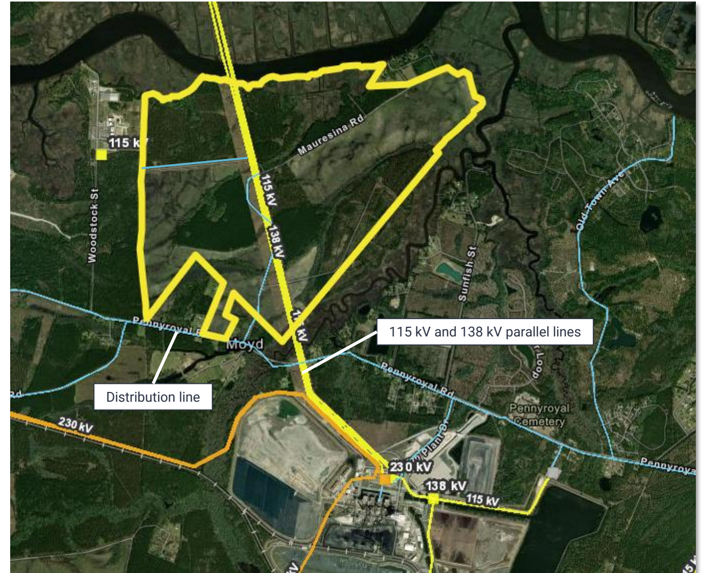
Electric & Natural Gas Infrastructure
