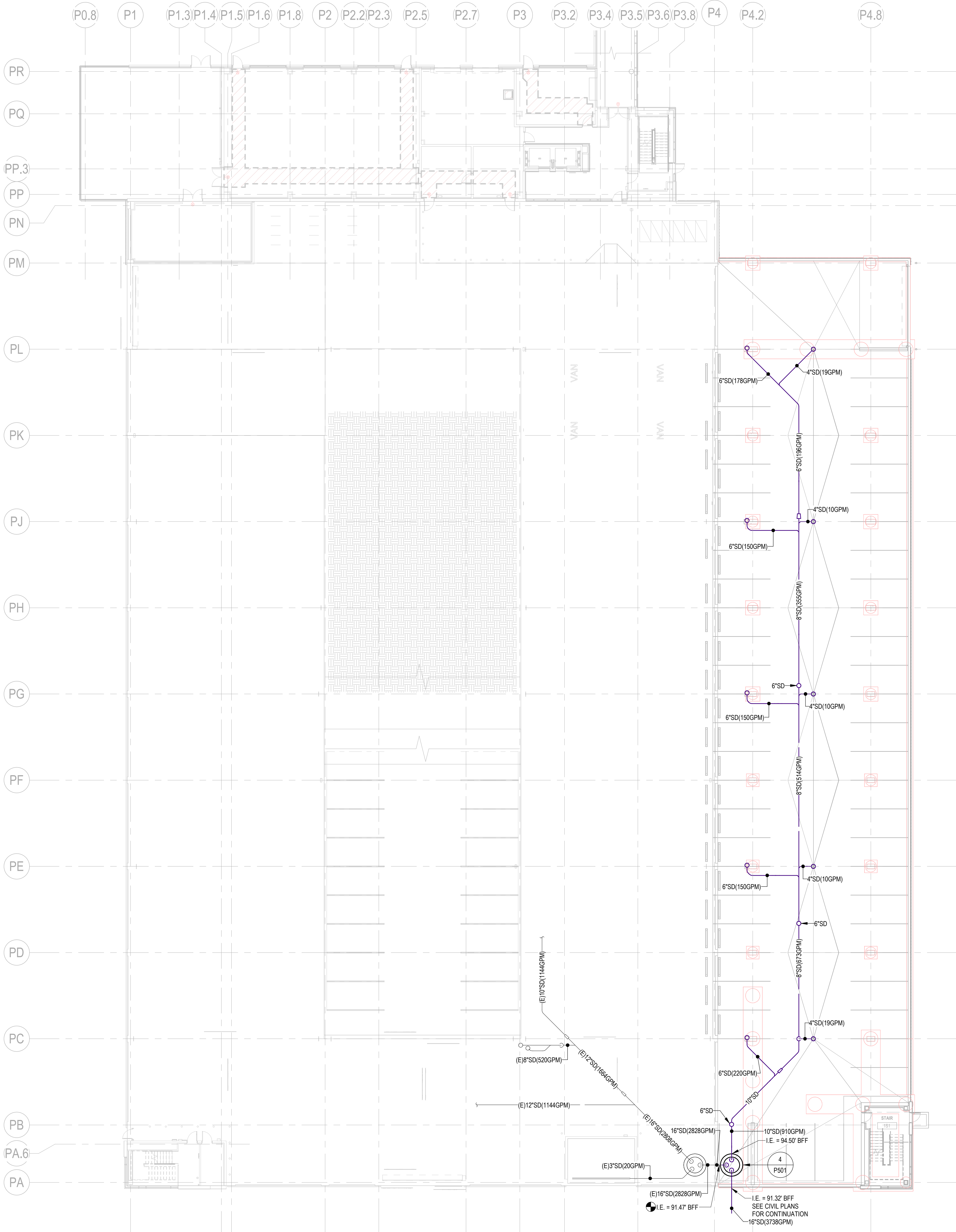
1 UNDERGROUND PLAN - PLUMBING 1/16" = 1'-0" NORTH 0 4 8 16 32
