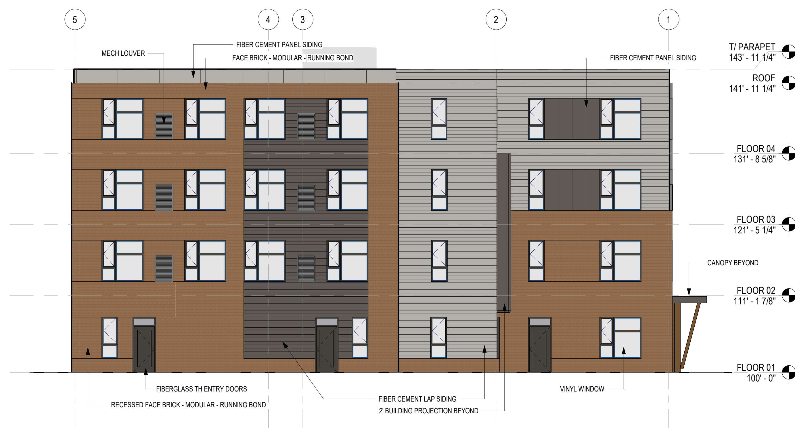
2 NORTH ELEVATION A200 1/8" = 1'-0"
