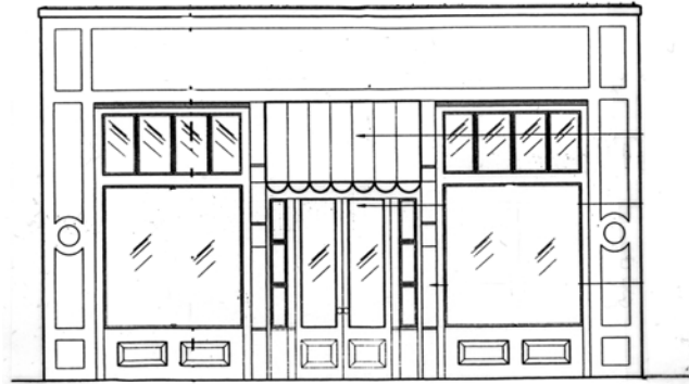
Inappropriate entrance design.
