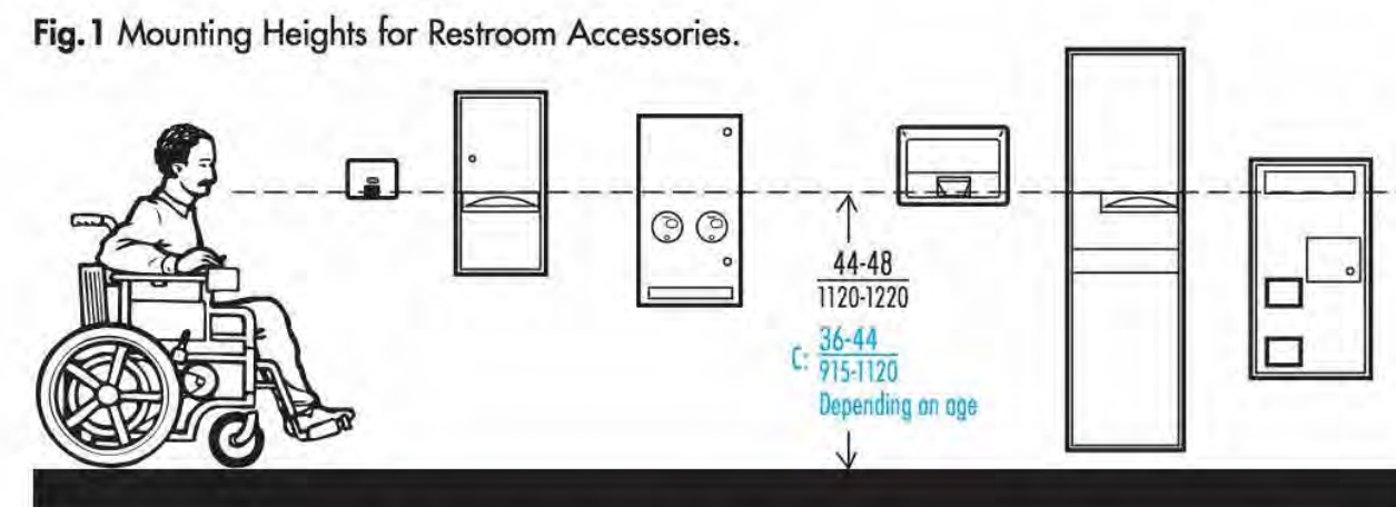
Fig. 1a Upper Range of Mounting Heights for Restroom Accessories with Operable Parts.
